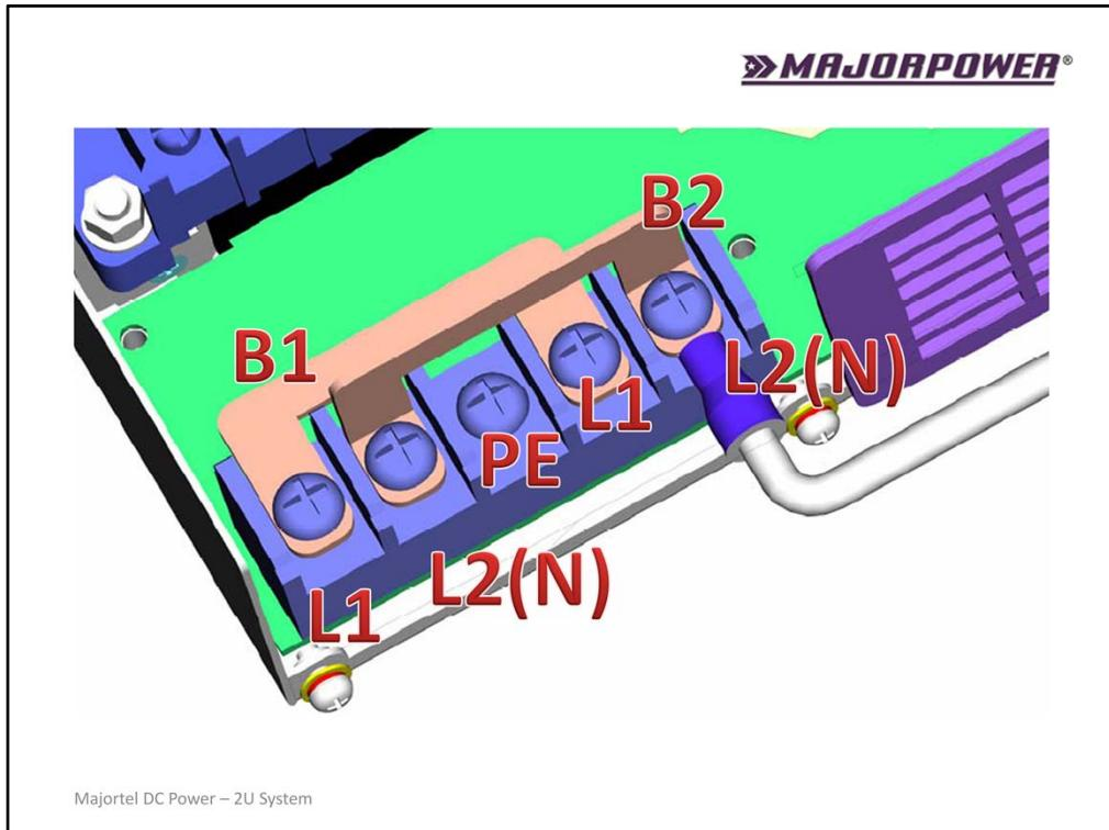
The Majortel 2U power system has the capability to accept AC input using a single or double power source.
